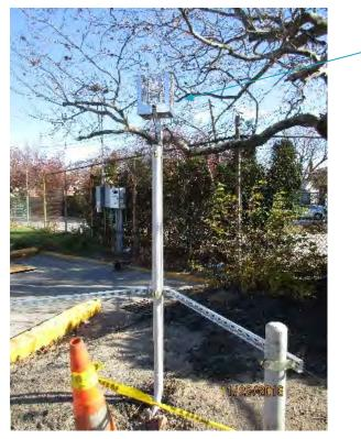
Photograph 2 – Solar powered wet sensor electronic housing
